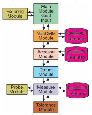
Figure 4 – Inspection Planning System Model
